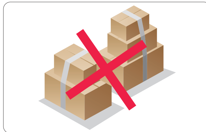
It is not possible to tie, tape, join by stretch foil or stick the consignments. Consignments attached to each other do not enable manipulation and can be torn.
